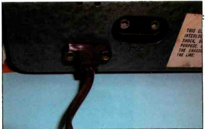
Photo K. The radio end of the cheater cord is riveted to the rear cover. (Photo Ed Engelken)
