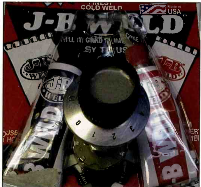
Photo C. JB Weld's self-leveling property is the key to repairing poke-through damage. Just keep the knob level as the JB Weld cures. (Photo Ed Engelken)
