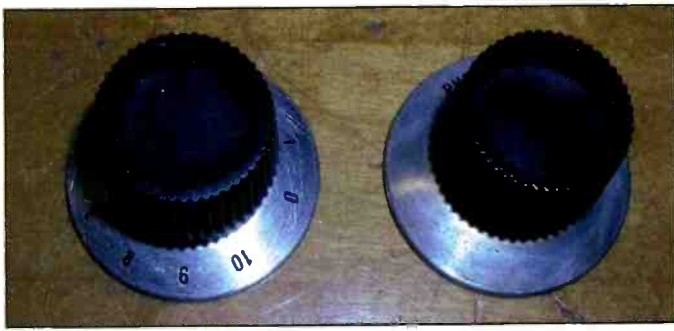
Photo D. The repaired knob on the left is difficult to distinguish from an undamaged knob on the right. (Photo Ed Engelken)
