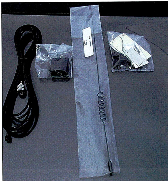
Here's the APR143 package: coax, inside coupler, the whip, and a small bag with the adhesive, grounding foil, and outside foot.
