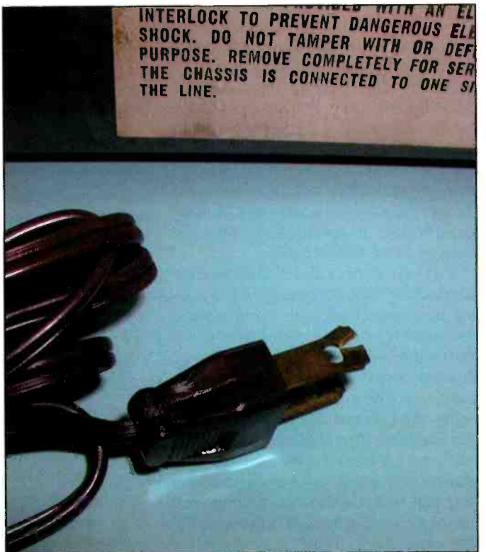
Photo L. Ed suggests this modification to make a non-polarized molded AC plug mate only with more modern polarized AC outlets. A pair of side-cutters is used to make one blade of the plug wider than the other. (Photo Ed Engelken)
