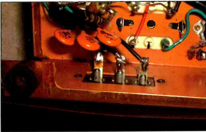
Photo I. These three capacitors, wired between the antenna and ground terminal strip and the bandswitch and chassis ground, serve to isolate the user from any dangerous AC voltages present on the chassis. They must be replaced with UL-rated line-bypass capacitors.
