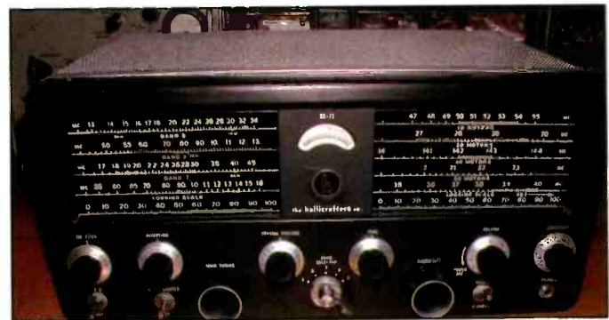
Photo G. The repaired/refurbished knobs, along with other repairs, have transformed the sad-looking SX-71 shown in Photo A into an attractive receiver. (Photo Ed Engelken)
