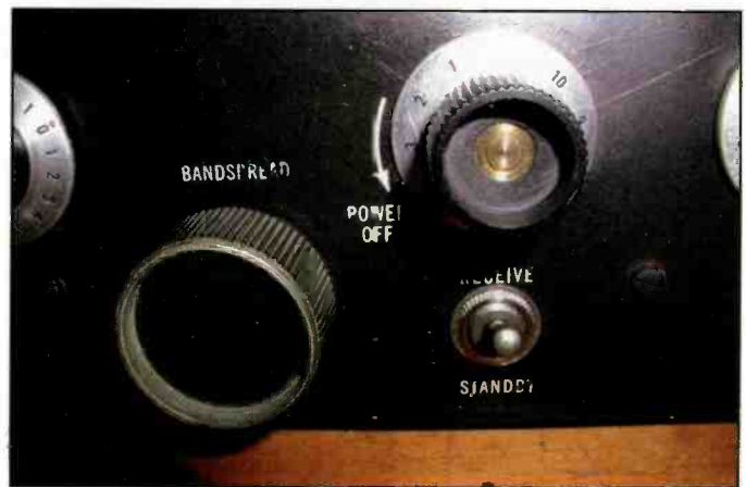
Photo B. Here's a typical example of poke-through knob damage caused by careless handling. Finding replacement knobs is difficult, so repairs are necessary. (Photo Ed Engelken)
