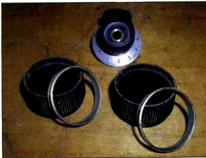
Photo E. The silver-painted brass “trim rings” in the large tuning knobs can be removed for repainting. Be careful when prying them out. (Photo Ed Engelken)
